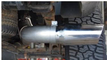
**Step 12** Orient the tubing so the hangers are secure and nothing contacts the exhaust. Pivot tube C so the exhaust tip is positioned straight and level.
