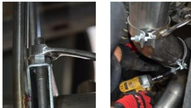
**Step 14** Tighten clamps (G, K), starting forward from the flange and moving back towards the tip (F), being careful that the exhaust is clear from contacting surrounding surfaces.
