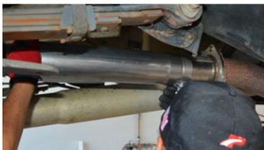
**Step 9** Feed the slotted end of tube B over rear axle. Install hanger bracket (D) over the slotted end of tube B. Feed hangers through rubber mounts to secure. Connect tube B to tube A and fit clamp (G) over the junction. Leave loose at this time.
