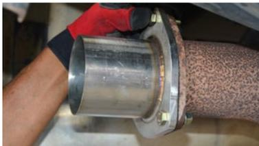
**Step 7** Fit one clamp (G) over the front slotted end of tube A. Fit tube A over the installed flange. Leave loose at this time.
