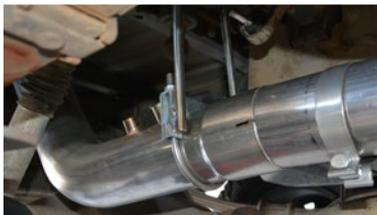
**Step 10** Install clamp with hanger (K) on the slotted end of tube C and fit over the rear end of tube B. Leave loose at this time. Feed hanger through rubber mount.
