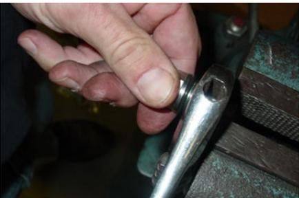
*Step 6. Another view of removing the valve cap after loosening in step 5.*
