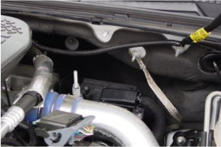
*Step 2. Remove the 5 bolts shown below. Remove black metal casing under bolts to access the Fuel Pressure Valve.*
