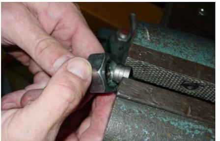
*Step 7. Remove the metal spring, then insert the two supplied metal shims into the valve. 3 shims are supplied with the DURAMAXIMIZER, however only 2 need to be used.*
