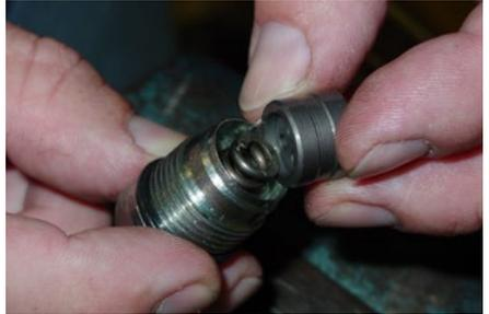
*Step 9. Place the valve back in the vice, now place a thick piece of cardboard (or piece of wood) behind the valve cap to prevent damage to the valve seal surface. Tighten the vice so that the valve cap re-enters the valve until fully seated. No need to overtighten, just tighten until snug.*
