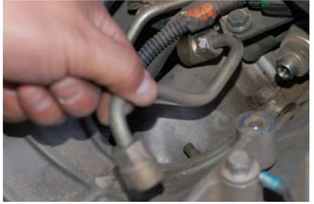
**Note: This fitting is in a tight spot. Quarter-turns of the wrench are required to remove this end of the line fitting.**
