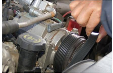
3. *Disconnect electrical connectors (shown in yellow) on the A/C compressor and set them to one side.*
