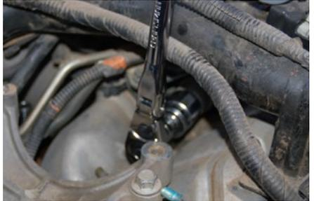
9. Lubricate the Ported Fuel Rail fitting with petroleum jelly, install and torque to 52 ft. lbs.
